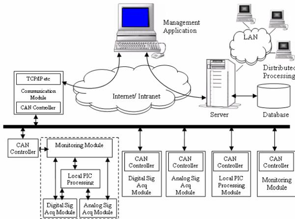
Fig. 1 Distributed monitoring system architecture
