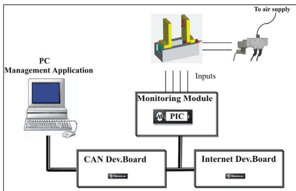
Fig. 6 Distributed monitoring system gripper Set-up
