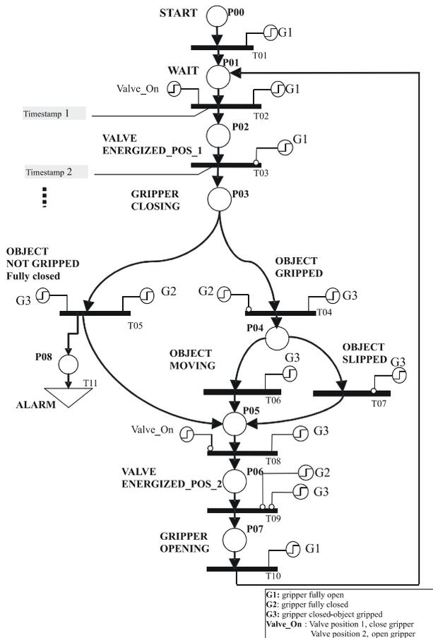
Fig. 5 Petri-net of gripper configuration with three limit switches
