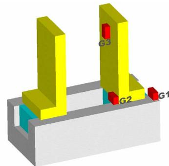
Fig. 2 Gripper configuration with three limit switches
