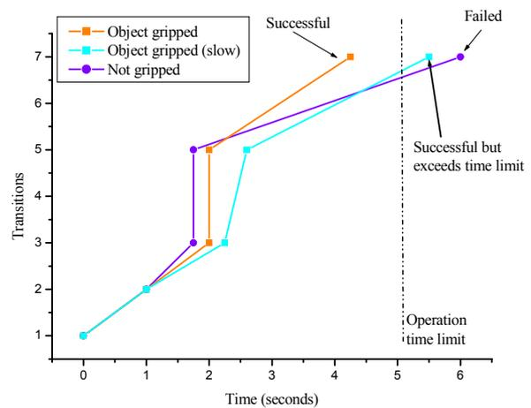
Fig. 7 Different timing results in a gripping operation
