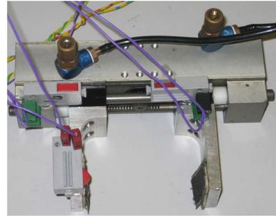
Fig. 4 Pneumatic gripper used in the lab
